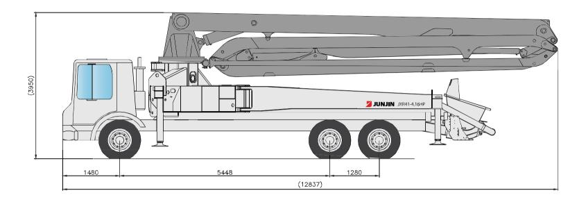
\* Remark: Standard specification with MACK 6X4. Dimension depends on truck specification.
