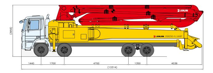
\* Remark: Standard specification with BENZ 8X4. Dimension depends on truck specification.
